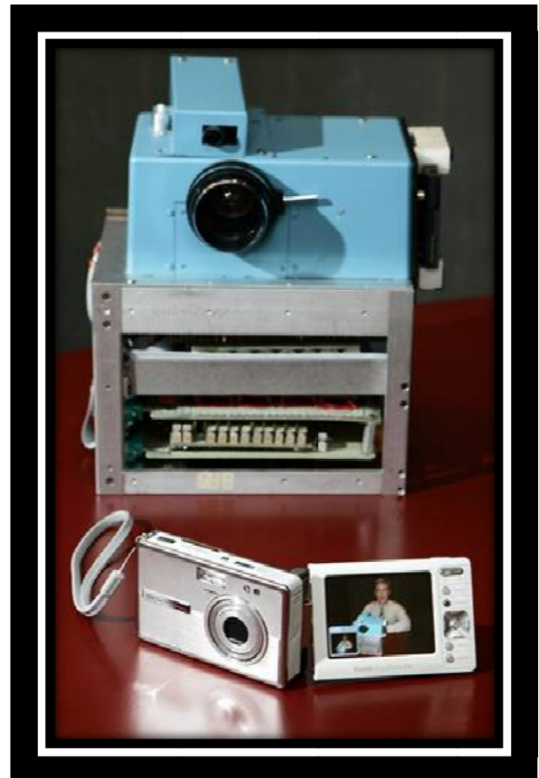
David Duprey / AP Kodak's prototype digital camera built in 1975 is shown next to Kodak's latest digital camera, the EasyShare One.
